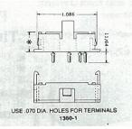
\*Socket may be soldered directly to PC board (O/A height \*=1.320") or snapped through underside of chassis. (O/A height = 1.208" when using recommended .062" chassis thickness).
